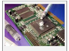
Ceramic-filled single component silicone with a high thermal conductivity.
