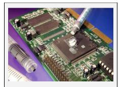
Ceramic-filled single component silicone with a high thermal conductivity.
