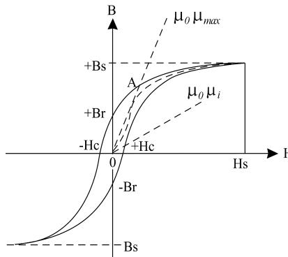
In the figure,  $B_S$  is saturation induction,  $B_r$  residual induction,  $H_C$  coercivity, and  $H_s$  saturation field.
