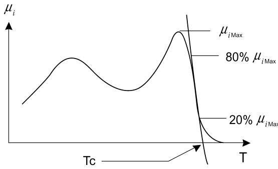
As temperature increases, one can find the two points with the permeability falling down to 80%  $\mu_{i\text{Max}}$  and 20%  $\mu_{i\text{Max}}$  respectively. Connecting the two points and extrapolating the line to T axis, the point of intersection is Curie temperature.
