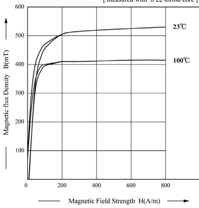
Saturation Magnetic Flux Density vs. Temperature
