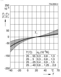
Initial permeability  $\mu_i$  and relative loss factor  $\tan \delta/\mu_i$  versus temperature (measured on R10 toroids,  $\hat{B} \leq 0.25$  mT)
