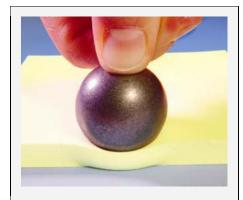
A group of highly elastic, ceramic-filled films. They are characterized by their excellent compressibility, their optimum plasticity with good thermal conductivity and good electrical properties. These films are especially suitable for compensating differences in planarity of the components or pressure sensitive applications.
