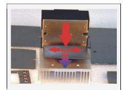
High density graphite with a very high thermal conductivity, as a cost-effective alternative to conventional heat spreaders. Up to 1/3 weight savings compared to conventionally used materials made from copper or aluminum. No electrical insulation!
