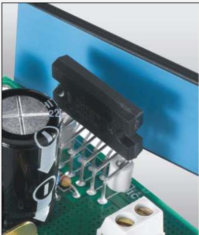
Thermoplastic elastomer tape with very good isolating behavior, excellent mechanical properties and good thermal characteristics
