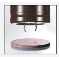
A new silicone-free Softtherm® film based on a copolymer. Besides good thermal behavior the film has good compressibility and aging resistance. This carrier-free film displays good relaxation behavior and can be produced in thicknesses from 0.5mm to 5.0mm.
