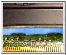
This group of Softtherm® films has a very good thermal behavior. The films are characterized by low thermal resistance and best heat dissipation, as well as good dielectric strength. Good compressibility and low shore hardness ensure reliable and simple processability.
