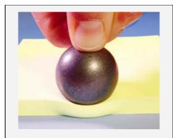
A group of highly elastic, ceramic-filled films. They are characterized by their excellent compressibility, their optimum plasticity with good thermal conductivity and good electrical properties. These films are especially suitable for compensating differences in planarity of the components or pressure sensitive applications.
